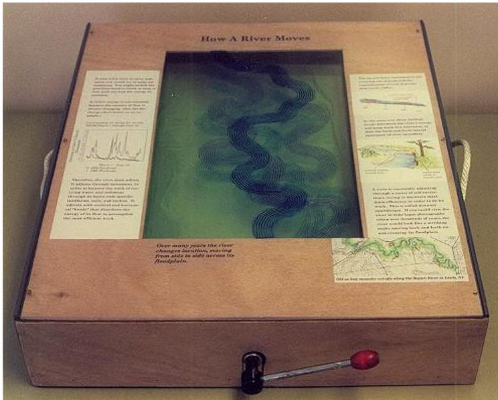
*Three plexiglass panels will move when the handle is pushed from side to side, making the river appear to writhe like a snake.*
