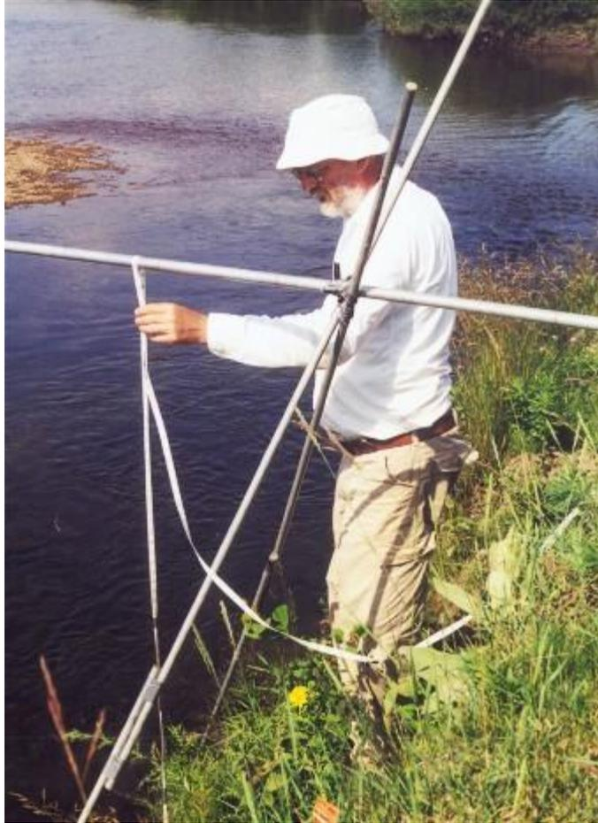
*Dennis Kalma measuring with plumbed tape off the ruled horizontal rod.*
