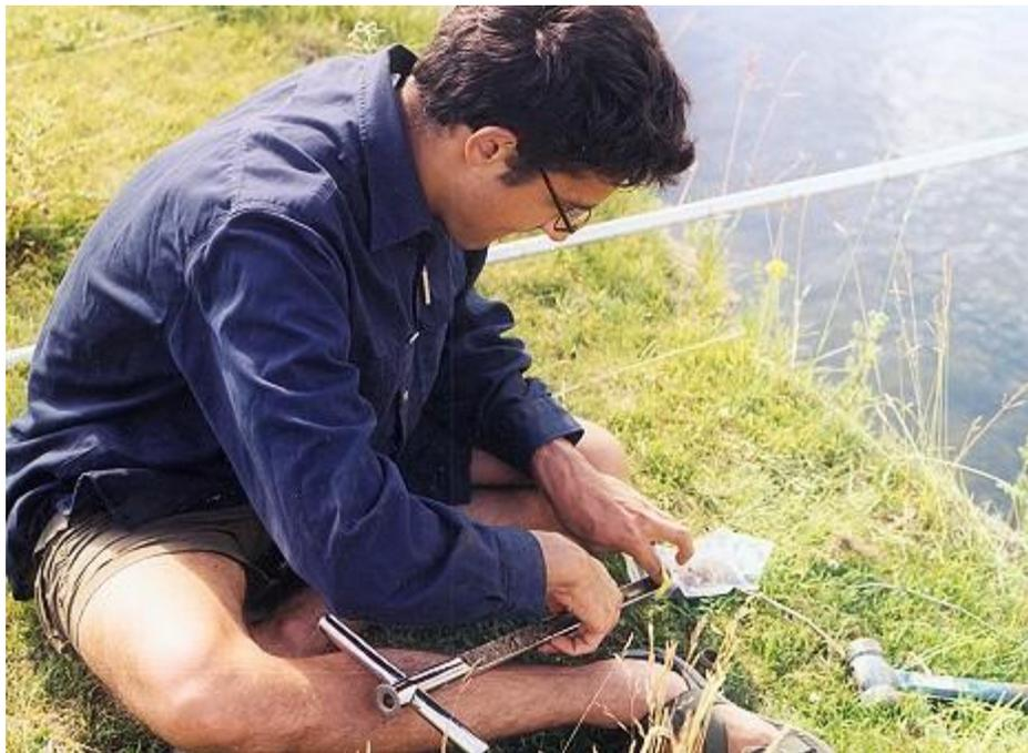
*Philip removes the soil sample into a pre-labeled plastic bag.*
