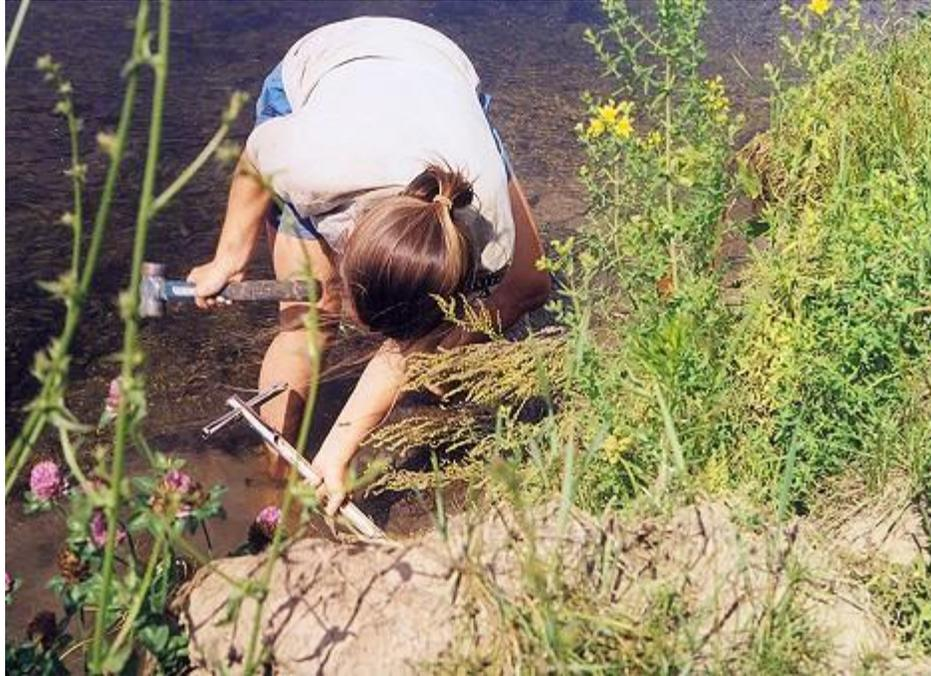
*Massey drives the soil sampler into the base of a streambank.*
